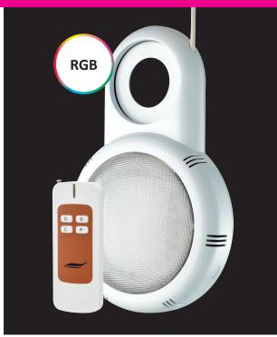
Model : **500699** Type : 36 LED 2835 / 120° Color : 12R, 12G, 12B Control : On/Off and 433Mhz radio remote Functions : 7 static colors and 3 programs Material : Fixture and lens in polycarbonate (PC), cover in ASA Fixing on 1,5" outlet fitting ~230V/~12V – 20VA plug transformer 6m HO5RNF cable 2x1mm<sup>2</sup> HS code : 9405403990 Bar code : 3700450500699
